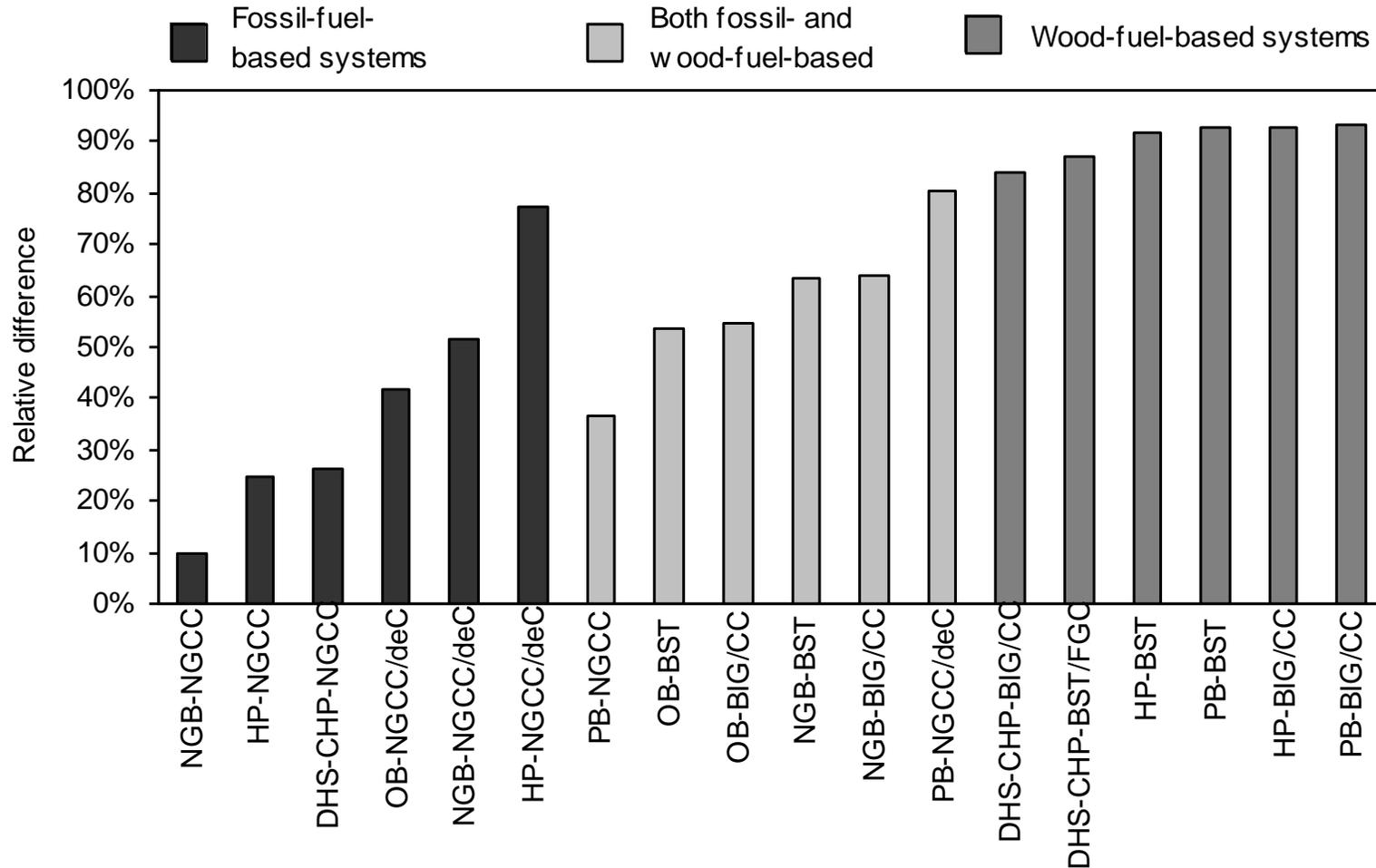
**CO<sub>2</sub> mitigation cost when the reference entity is produced in the energy systems and the oil-boiler system using NGCC is the reference. The cost of the reference system was €100 per reference entity**
