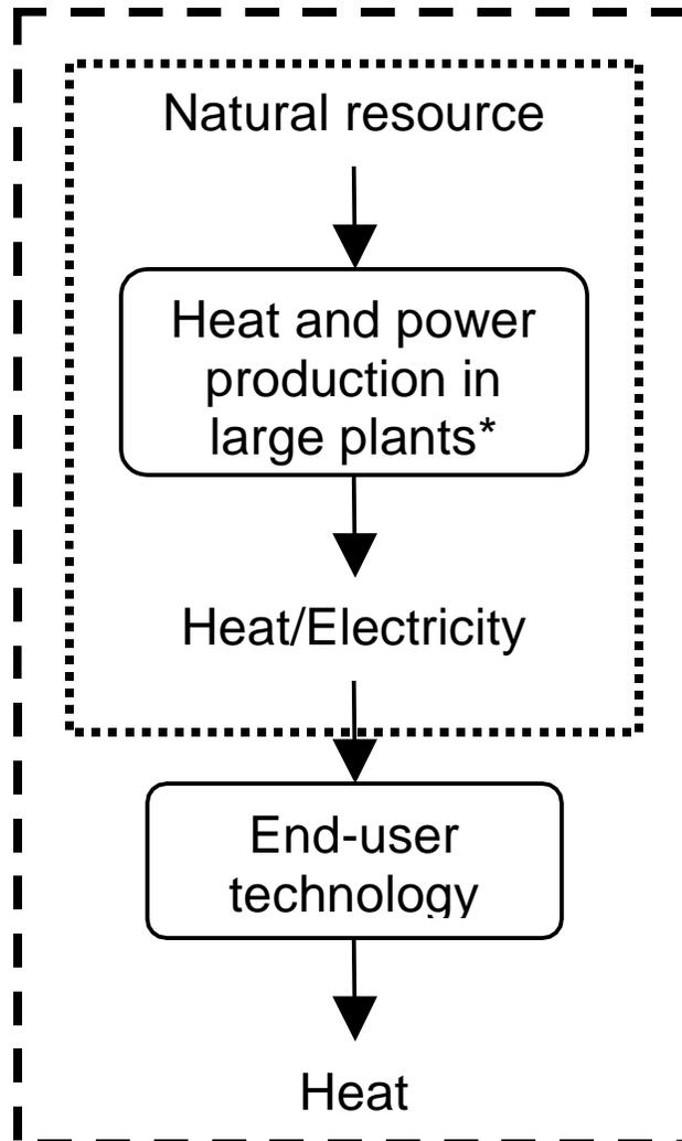
The dotted line shows the boundaries of the large-scale system..The dashed line shows the boundaries of the total system for district heating and electric heating systems. In the local boiler systems, the large systems are used for producing the electricity input only.
