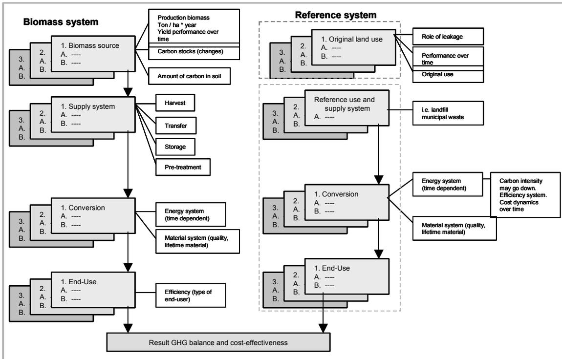
Figure 2: Flow chart design for software tool BIOMITRE
